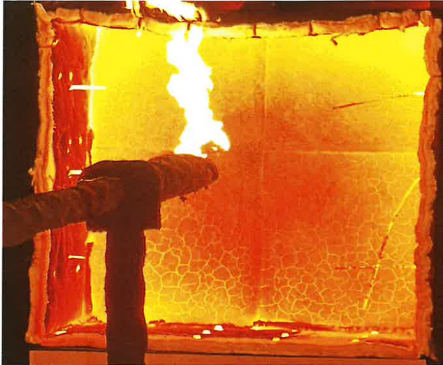
Figure 8: Close up showing condition of exposed face just after fire exposure: Cracking pattern on the surface is visible
