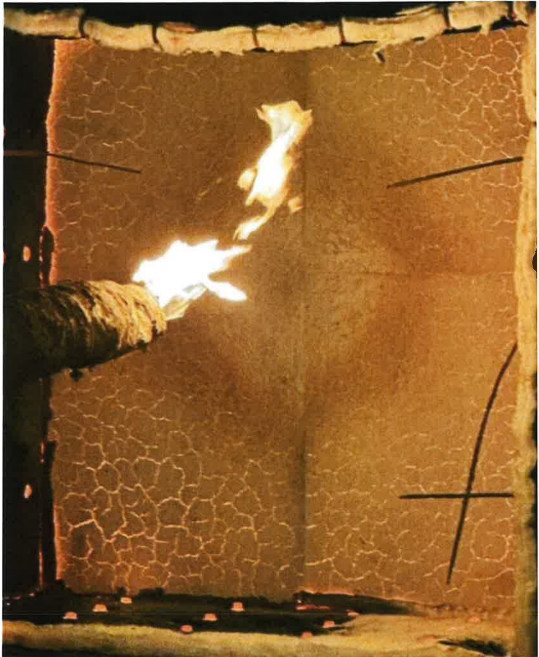
Figure 10 Close up showing condition of exposed face of the specimen during cooling.
