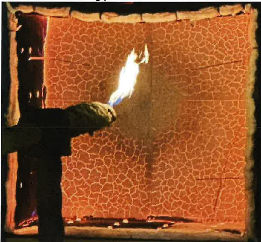
Figure 9: Close up showing condition of exposed face after few minutes of shutting off the burner
