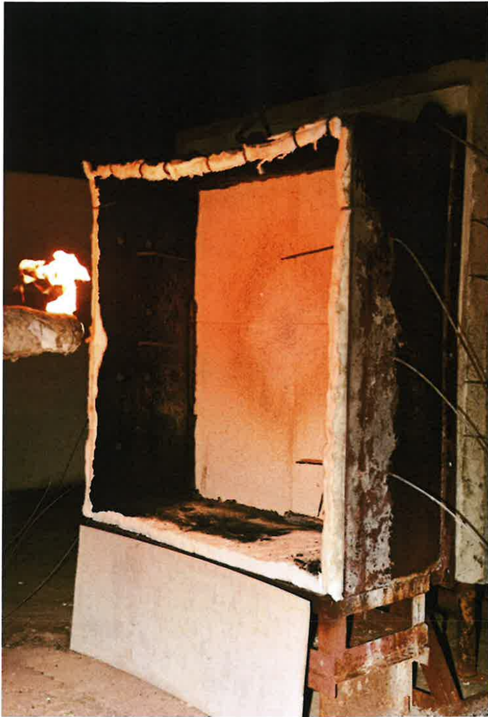
Figure 7: Close up showing condition of exposed face after fire exposure
