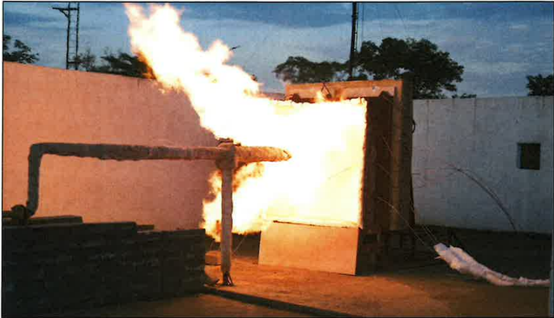
Figure 1: Jet fire resistance test at Amguri field, Assam
