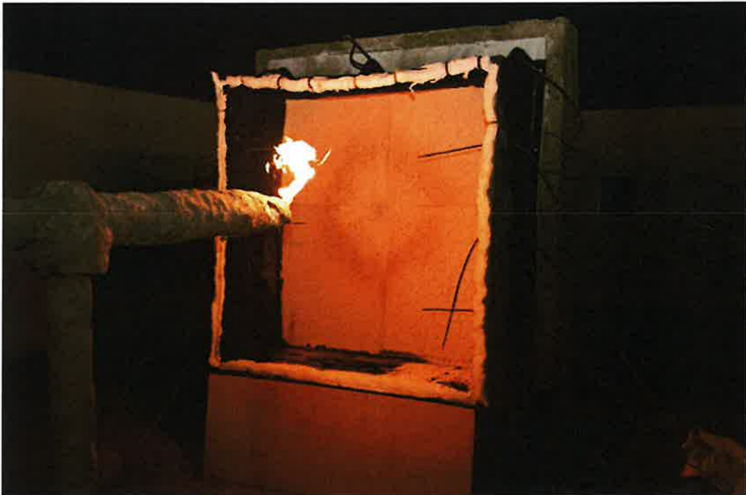
Figure 6: Condition of exposed face after fire exposure
